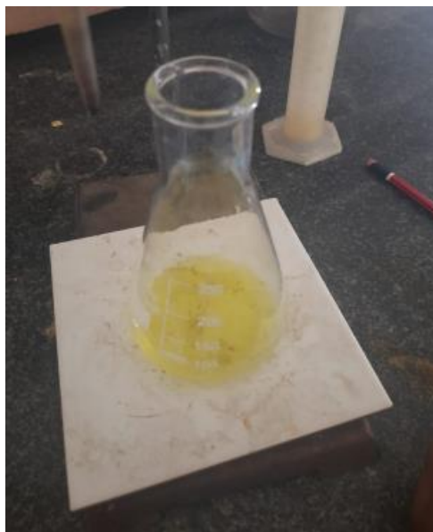
Starting point of chloride
