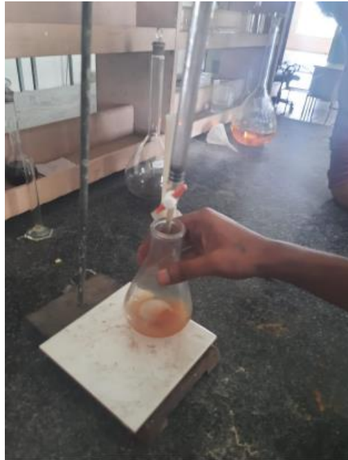
End point of chloride
